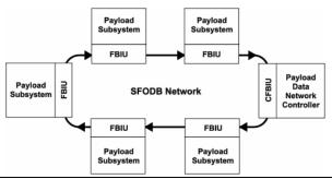
The CFBIU provides the network management and data routing functions that allow each FBIU to transport data in one of four methods: dedicated transmit, dedicated receive, tokenized transmit, and ATM Header addressing. The network has an additional Bandwidth Reuse feature that allows the network to operate in a segmented ring configuration. This feature allows a user to multiply the data handling capacity of the SFODB network by the number of ring segments implemented<sup>3</sup>.
