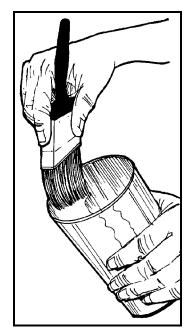
Figure 7. Pushing Brush Against Inside of Container.
