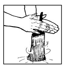
Figure 6. Removing Loose Bristles.
