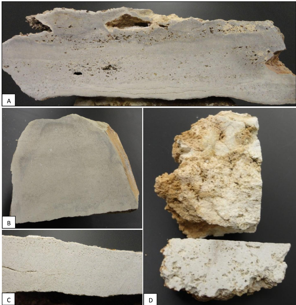
Figure 7: Photos of cut hand samples. A) Bed 6, vugs and matted bedding. B) Bed 3, no internal structure or vugs. C) Bed 7, shows how porosity increases on the exterior where weathering occurs (weathering rind). D) Bed 4, loosely compacted and high number of large vugs.
