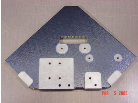
**Figure 13. Top Deck Test Coupon**
