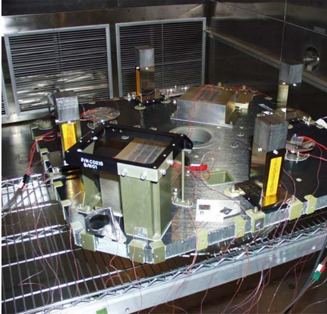
**Figure 16. Bottom Deck Thermal Cycle Test**
