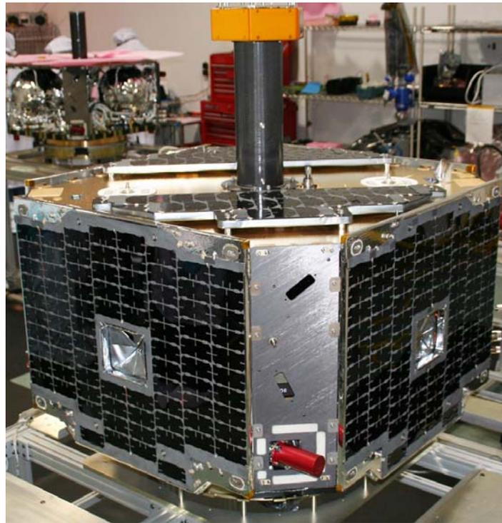
**Figure 5. Probe Bus External Photo**
