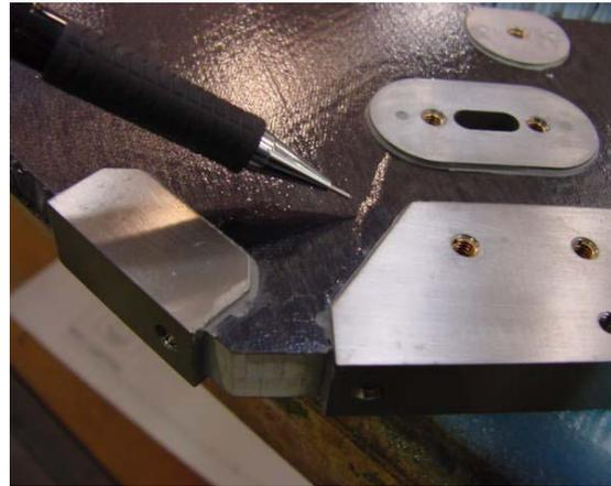
**Figure 11. Top Deck Face Sheet CTE Failure**
