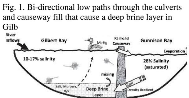
Fig. 1. Bi-directional low paths through the culverts and causeway fill that cause a deep brine layer in Gilbert
