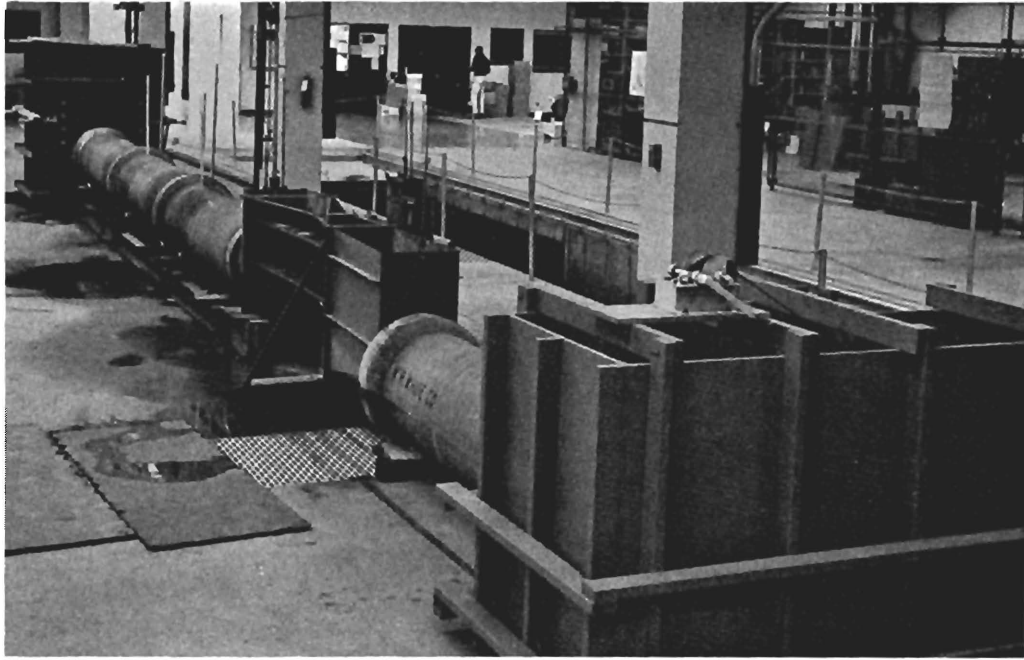
Figure 2. Oblique view of the experimental arrangement for the 9-inch Parshall flume.
