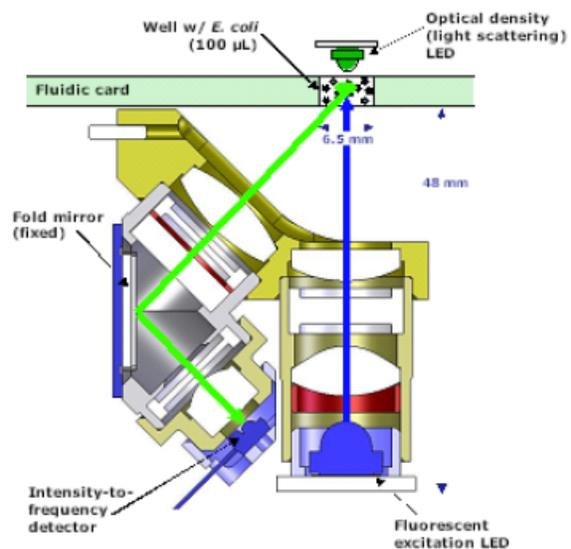
Figure 5 – The Payload Optical Detector System
