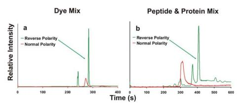
Fig. 6 Representative electropherograms of the separations performed with CE on a PEG coated fused silica capillary with reduced EOF. Two injections using opposite polarities between the separations are required because of the reduced EOF. In (a), the separation of the fluorescent dye mixture is shown, and in (b), the separation of a protein and peptide mixture is shown.
