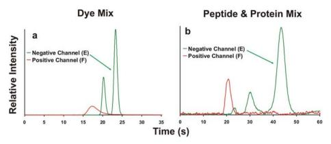
Fig. 4 Representative electropherograms of the separations performed on the PEG coated (low EOF) microfluidic device. Sample injection from a central channel is achieved, and anions and cations are separated in different channels. An electropherogram of the fluorescent dye mixture is shown in (a), and an electropherogram of the protein and peptide mixture is shown in (b). Each component was baseline resolved with high efficiencies in <1 minute.
