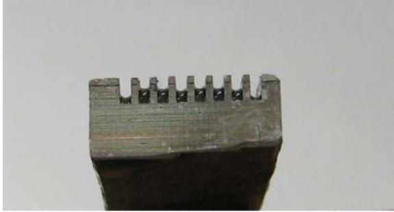
**Figure 8. Multiple menisci formed with isopropanol in sealed aluminum grooves.**
