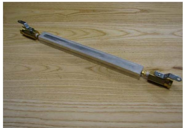
**Figure 10. Completed proof of concept heat pipe with fill valves.**
