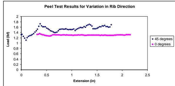
**Figure 3. Effective peel strength from a typical peel test.**
