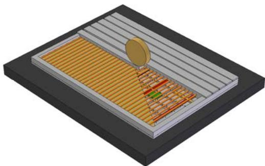
**Figure 1. Manufacture of a multipurpose structural panel using ultrasonic consolidation.**
