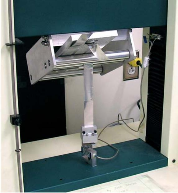
**Figure 2. Testing the ultrasonic bond through a peel test of a tape bonded to a rib structure.**
