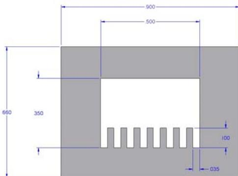
**Figure 9. Cross section of proof of concept heat pipe.**
