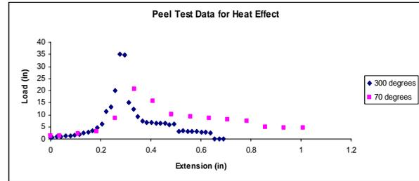
**Figure 4. Peel strength data when tape tears while peeling.**
