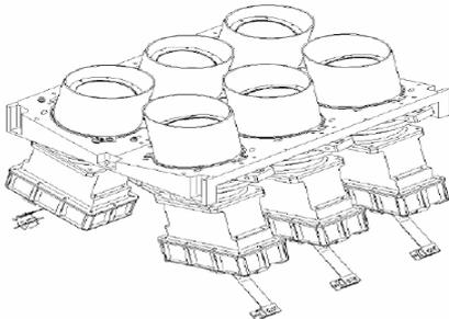
**Figure 1. Dual Bank DMC Channel Pairs**
