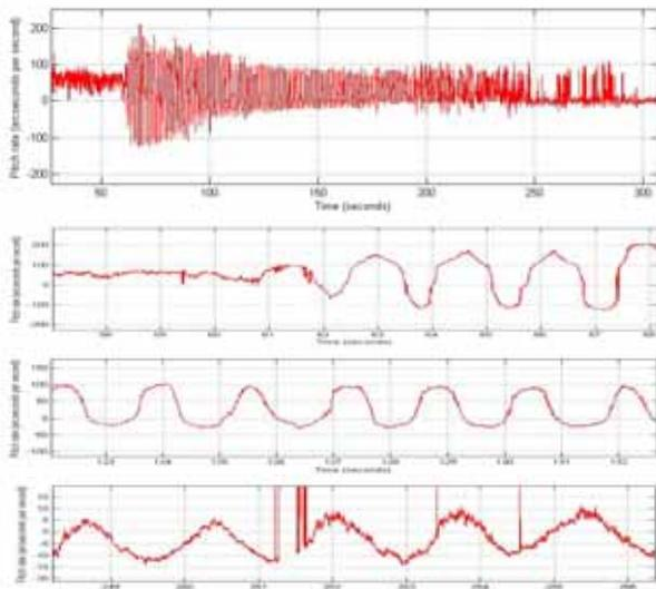
**Figure 11. Effect of y-axis Momentum Wheel Activation**
