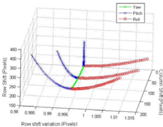
**Figure 5. Effect of consecutive yaw, pitch and roll on inter-image geometry**
