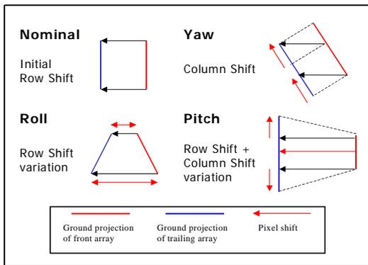
**Figure 4. Effect of attitude position on ground projection of alternate imaging arrays**
