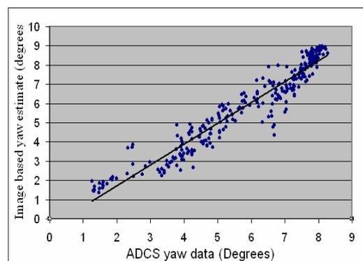
**Figure 13. Correlation between Estimated and ADCS Yaw Data**
