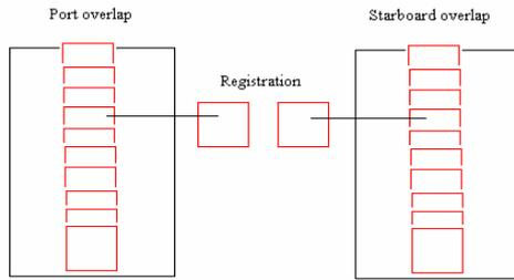
**Figure 7. Registration of DMC image segments**
