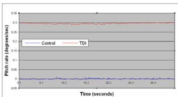
**Figure 8. Pitch Rate of Stationary and Rotating UK-DMC as Extracted from Imagery**
