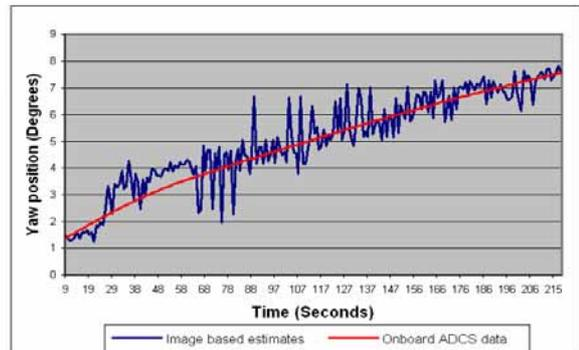
**Figure 12. Actual Drift in Yaw Vs Image-based Estimates**
