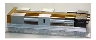
Figure 8. Breadboard model of optical correlator
