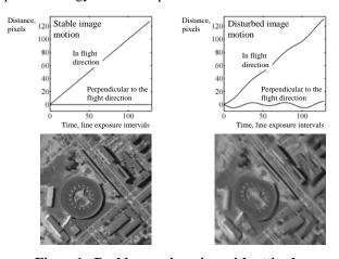
Figure 1. Pushbroom imaging with attitude disturbances
