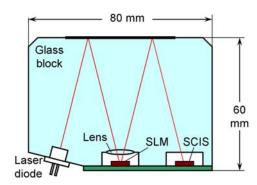
Figure 9. Advanced optical system layout
