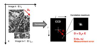
Figure 6. Image shift vector determination by 2D correlation
