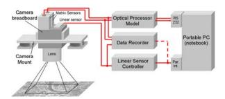
Figure 11. Test equipment configuration onboard the plane
