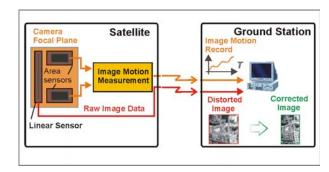
Figure 3. SMARTSCAN system concept
