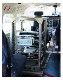
Figure 13. Test equipment mounted onboard the plane
