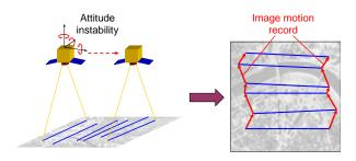
Figure 2. Disturbed pushbroom imaging and image motion record
