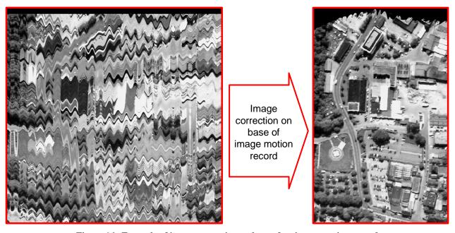
Figure 16. Example of image correction on base of an image motion record
