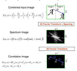
Figure 7. Principle of joint transform correlation
