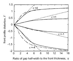
FIG. 3. Front profile distortion  $\Gamma$ , defined as the ratio of the front height to the width, vs  $\eta$  for  $\epsilon$ = -4, -1, 1, and 4. The results from the full advection-diffusion-reaction equation are shown with the solid trace, from the eikonal equation with the chain-dashed trace, and from the small- $\eta$  analytical curve with the dashed trace.
