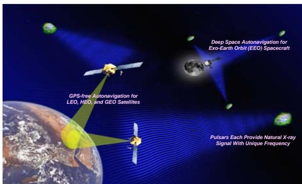
**Figure 2-1 Potential XNAV Mission Concept of Operations (CONOPS) <sup>4</sup>**
