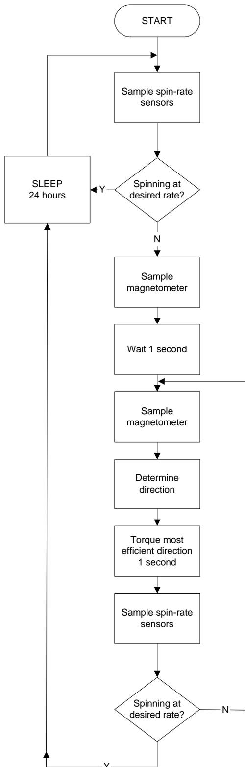
**Figure 9. High-level flowchart of the DISCO magnetic spin-rate controller software for STARSHINE 4. Each block represents a module called by the main control routine.**
