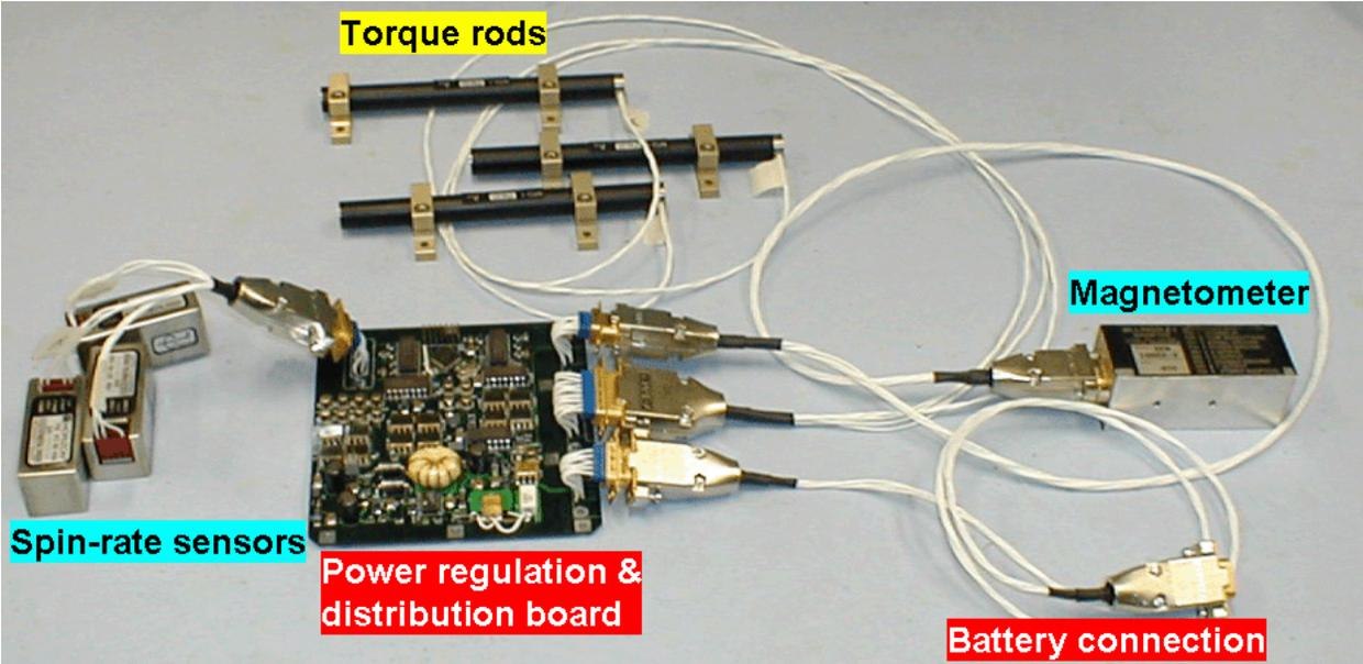
Figure 7. Complete DISCO system, including spin-rate sensors, torque rods, magnetometer, custom power regulation and distribution board populated with electronic components, and battery connection.
