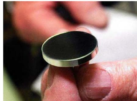
**Figure 2. Polished aluminum mirror prior to mounting on STARSHINE satellite.<sup>2</sup>**
