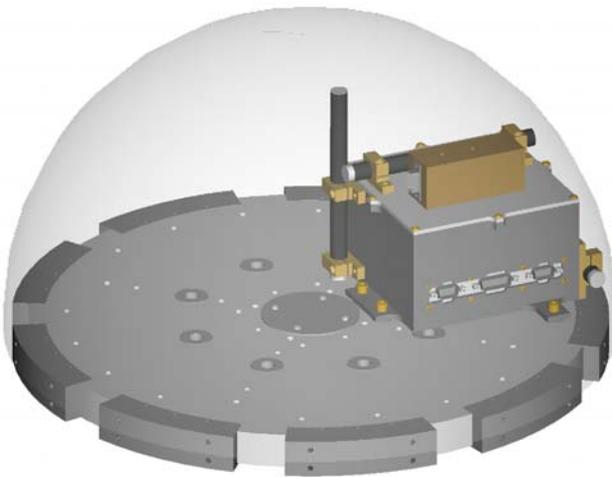
**Figure 10.** Rendering by Adam Webster, UND post-graduate mechanical engineering research assistant, of the DISCO enclosure mounted to the central deck of STARSHINE 4.
