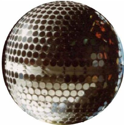
**Figure 1. STARSHINE 1, covered with nearly 900 polished circular aluminum discs.<sup>2</sup>**
