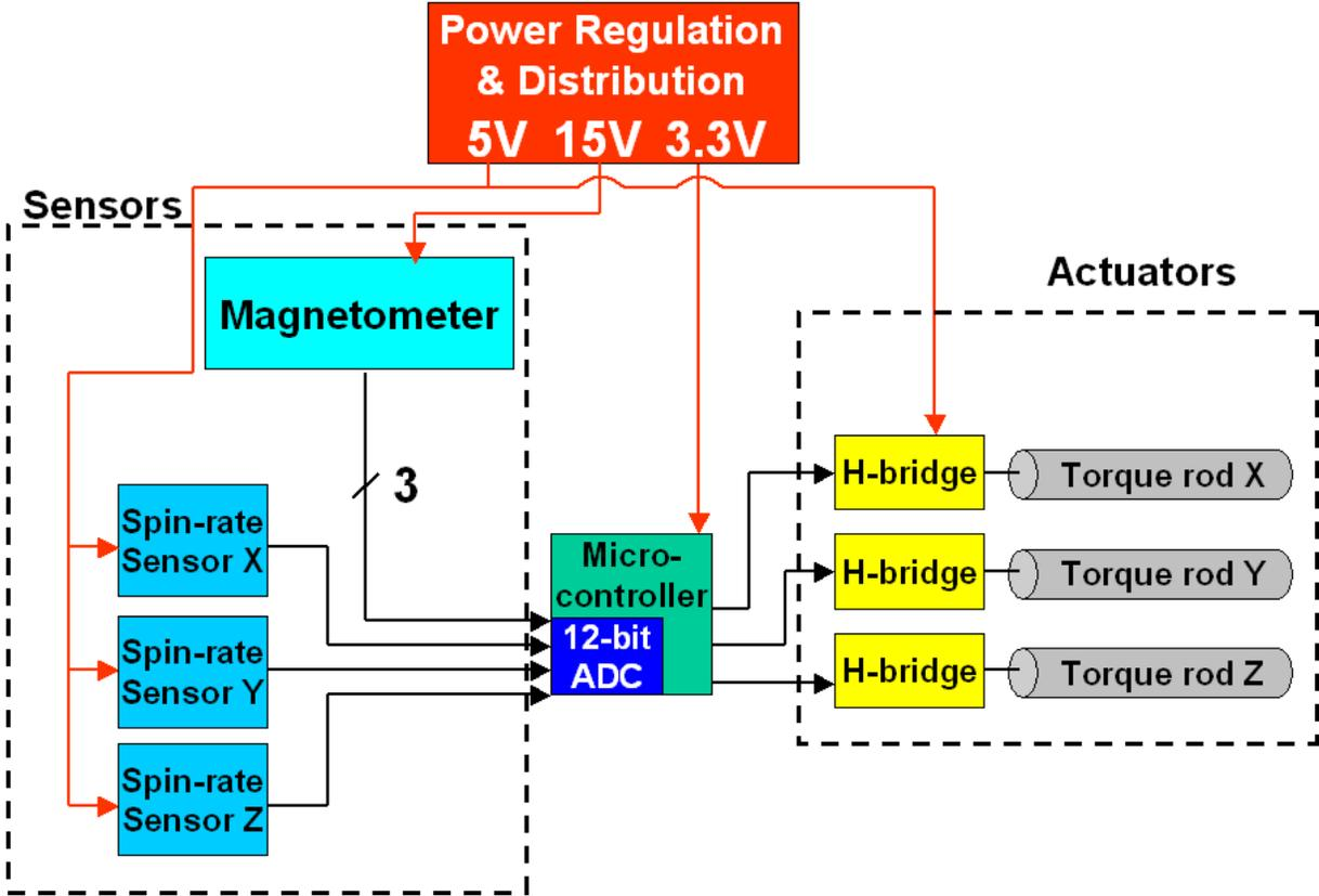
Figure 6. DISCO magnetic spin-rate controller system hardware component block diagram.
