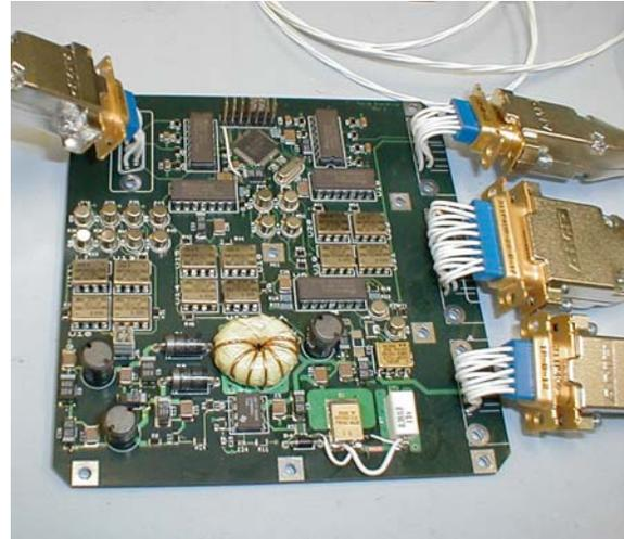
**Figure 8. Custom-designed power regulation and distribution board.**
