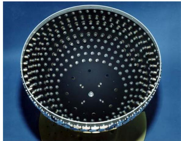
**Figure 12.** Interior of a STARSHINE satellite, showing the individual mirror mounting.<sup>2</sup>
