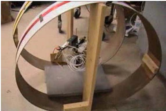
**Figure 13. DISCO system suspended by fishing line, undergoing a test in the Helmholtz coil electromagnetic field.**
