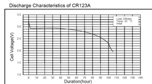
**Figure 15. Battery discharge characteristics (four cells will be used in series to ensure that voltage levels stay above 9 VDC for the duration of the mission).**
