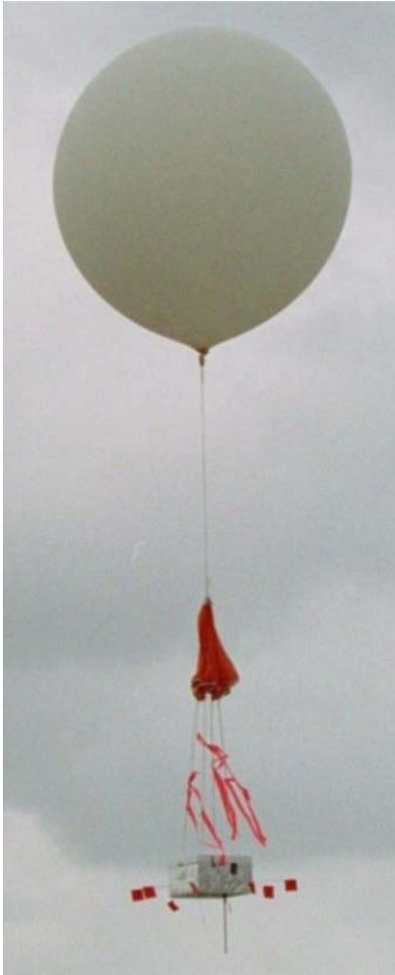
**Figure 3. The Instrumentation Platform is being launched using a burst balloon, during one of its test flights in Upstate**
