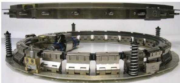
**Figure 2. A separation system: The Lightband**
