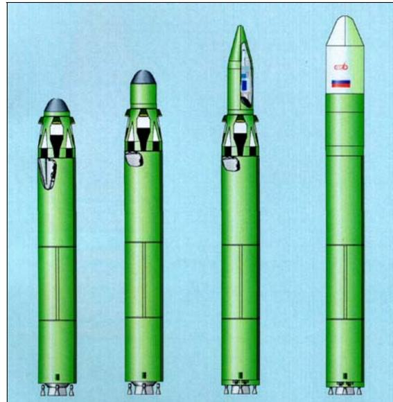
**Fig. 6. The ‘Shtil’ family of launch vehicles converted from the SS-N-23 (RSM-54) SLBM, from left to right: ‘Shtil-1’, ‘Shtil-2.1’, ‘Shtil-2’, ‘Shtil-3’**
