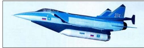
**Fig. 9. A model of the 'Ishim' launch system's MiG-31I carrier aircraft with a suspended launch vehicle**
