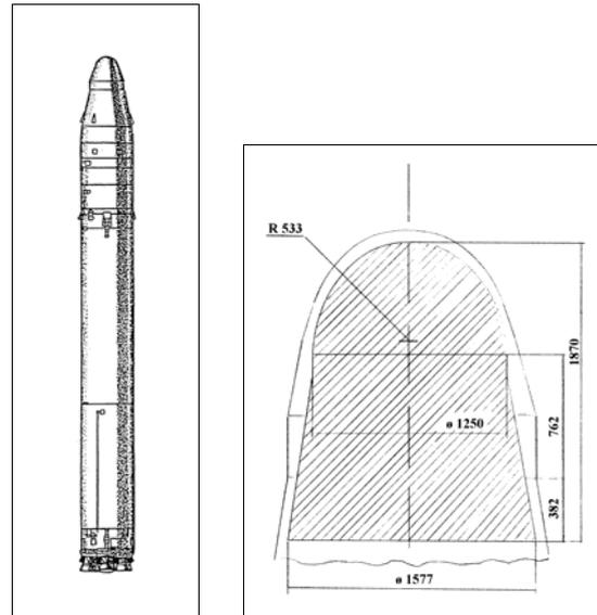
**Fig. 2. The general configuration of the ‘Rockot’ launch vehicle’s early silo-based version (left) and its payload accommodation zone (right)**
