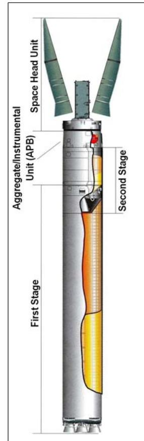
**Fig. 3. The design of the ‘Strela’ launch vehicle**
