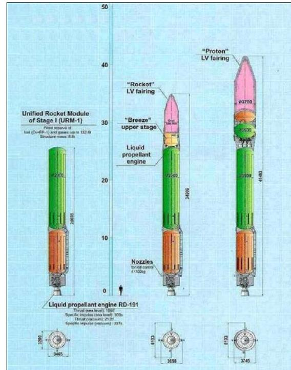
Fig. 8. Designs of the URM, 'Angara-1.1' and 'Angara-1.2' (left to right)
