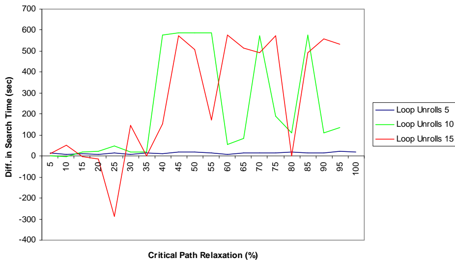
Fig. 5.6: Difference in the search time of version 1 and version 2 of the constraint solver for the DCT data flow graph.
