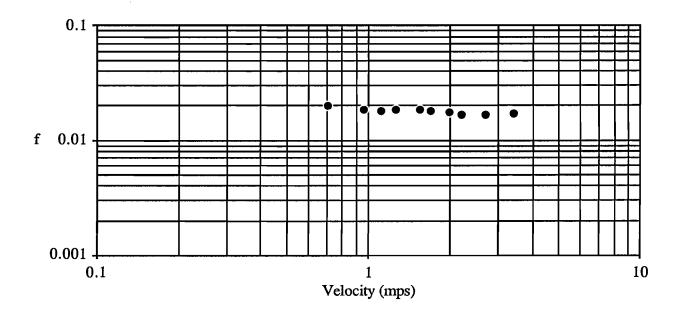
Friction f vs. Velocity for 375mm Diameter HDPE Pipe Figure 3
