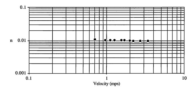
Manning n vs. Velocity for 375mm Diameter HDPE Pipe Figure 2
