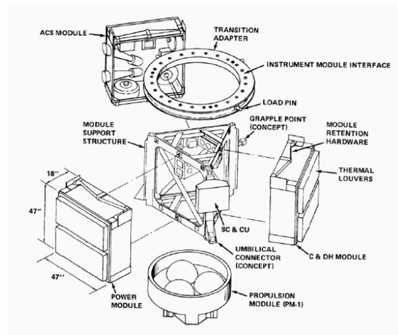
**Figure 4. NASA GSFC Multimission Modular Spacecraft<sup>20</sup>**
