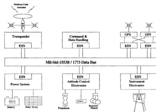
**Figure 5. NASA GSFC Modular Essential Services Node (ESN) provides a common interface for the data network.<sup>21</sup>**
