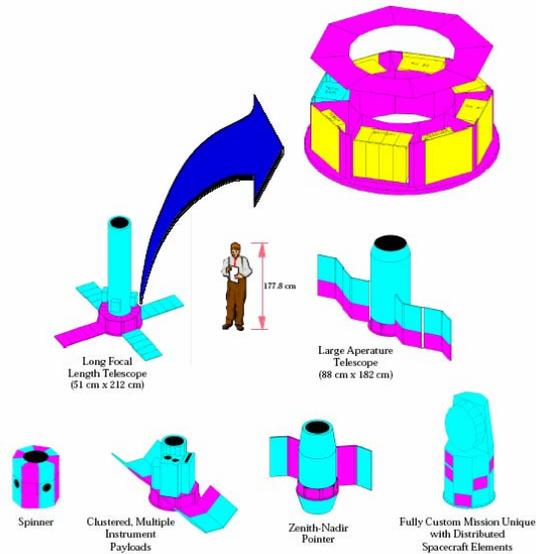
**Figure 3. NASA GSFC SMEX-Lite platform as a modular component of satellite observatories<sup>19</sup>**
