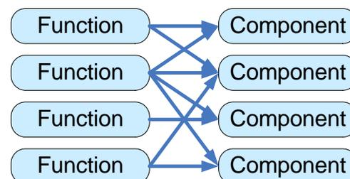
**Figure 1. Integral architecture**
