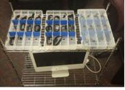
Fig. 3. Custom cart for storing, charging, and syncing a classroom set of 30 Fitbits devices when they are not used by students. Having such a cart is important in classroom contexts where class sets of equipment need to be mobile so they can be transported quickly.
