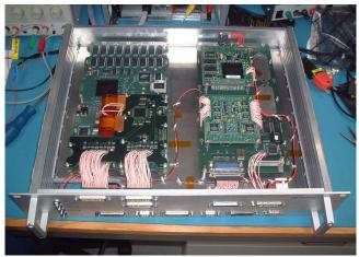
On left: SSTL SSDR assembly. On right: router assembly. **Figure 2. Ground-based testbed**
