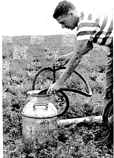
Fig. 6. Method of obtaining nozzle discharge volumetrically, using \frac{3}{4} -inch rubber hoses and a 10-gallon can
