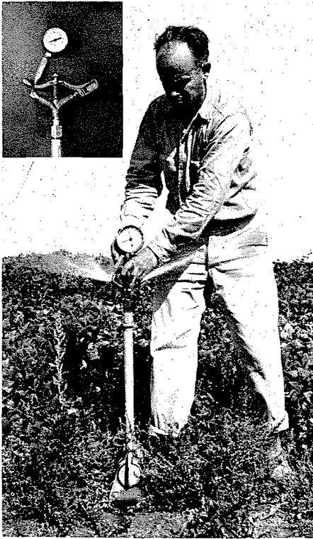
Fig. 5. Method of measuring nozzle pressure with a pressure gage and pitot tube attachment
