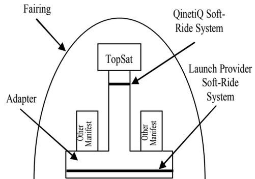
Figure 6. Test configuration for the QinetiQ anti-vibration system
