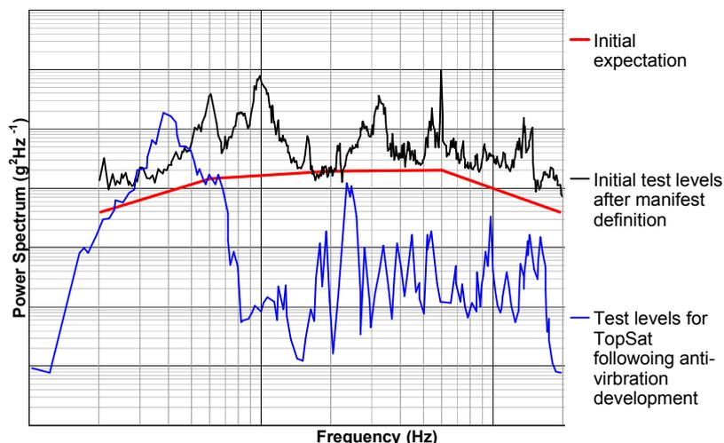
Figure 7. TopSat launch spectrum
