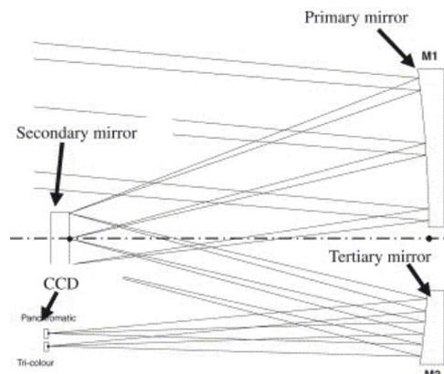
**Figure 3. The TopSat camera optical path**
