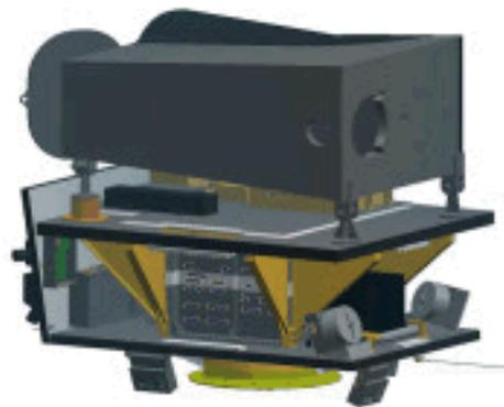
**Figure 2. The TopSat spacecraft showing the structure, bus and payload**
