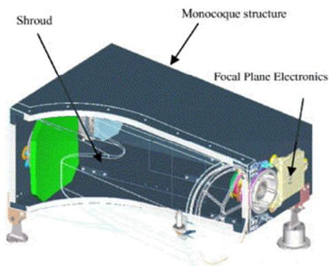
**Figure 4. The TopSat camera**
