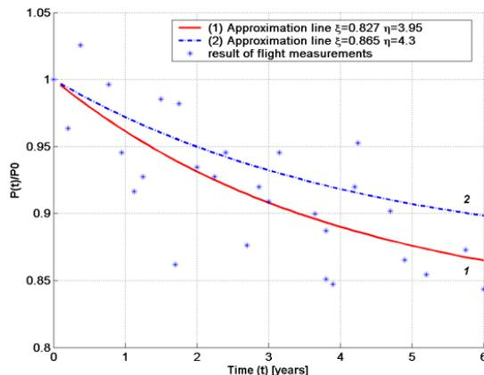
**Figure 5. Solar Arrays of silicon cells degradation during long-term space tests (curve 1 – LEO Techsat, curve 2 – GEO)**
