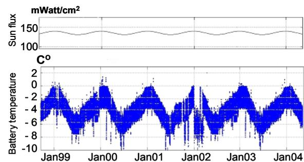
**Figure 6. In orbit electric battery temperature measurements and Sun flux variation during 1998-2004.**
