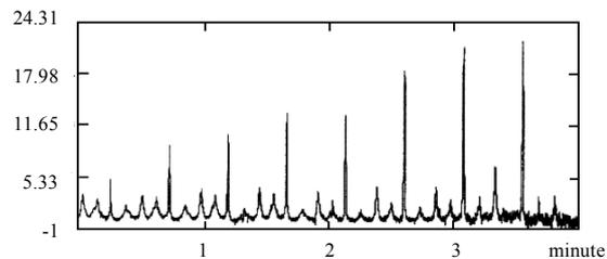
**Figure 9. The Brightness Curve of TechSat satellite during an observation session (in stellar magnitudes).**
