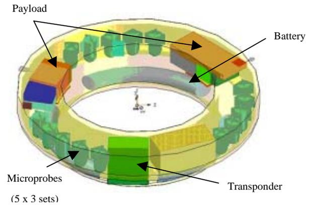
Figure 4 Gondola Internal Configuration
