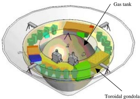
Figure 4 Gondola within Aeroshell
