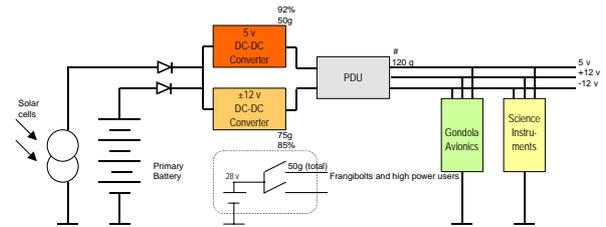
**Figure 7 Topology: Primary battery with solar array**
