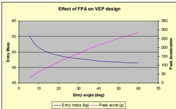
Figure 3 Effect of FPA on VEV Design
