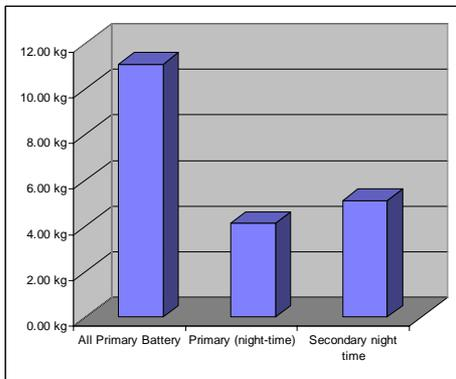
**Figure 6 System mass comparison of three alternative topology options for 30-day operational lifetime**
