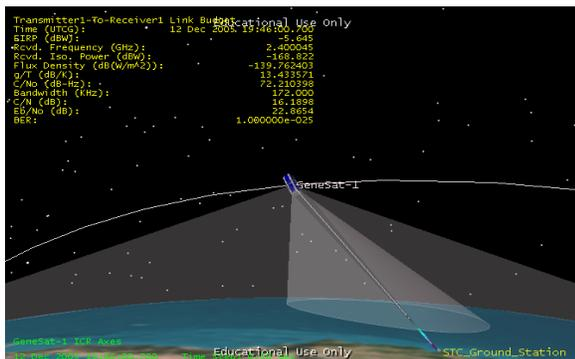
**Figure 29: 10-meter Dish Link Budget Using the Monopole Antenna**
