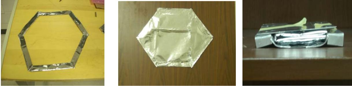
Figure 5. Replica ballute outer torus ring: Six strut-shaped mylar pouches attached with epoxy (left); Hexagonal ballute attached with epoxy to these pouches (center); Stowed hexagonal ballute in prototype storage bin (right).
