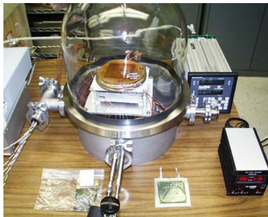
**Figure 7. Electrochromic device calorimetric test apparatus (Jet Propulsion Lab)**
