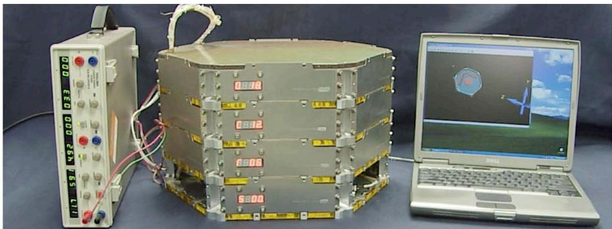
**Figure 5. An Assembled, Functional SMARTBus Stack with Ground Support Equipment.**
