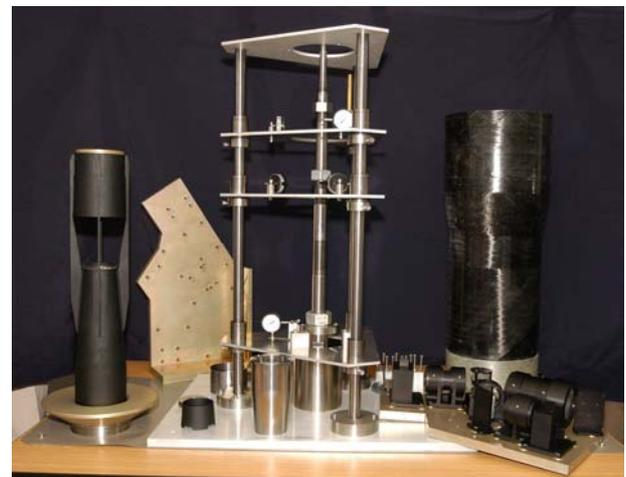
**Figure 12: Optical Assembly Jig (centre) with the Central Optical Element Structure (left), Outer Telescope Baffle (right) and Hyperspectral Unit (right front).**
