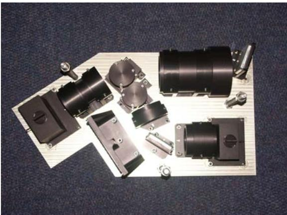
**Figure 11: Structural Model of the Hyperspectral Sensor Unit**
