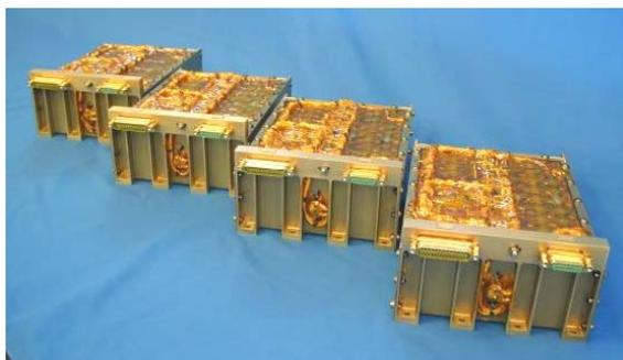
**Figure 1 The Qualified 28V 15Ah Module**
