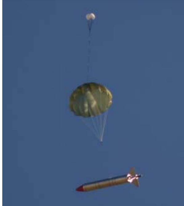
**Figure 4. Successful P-5 Parachute Deployment**
