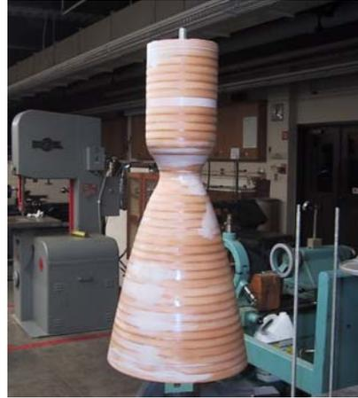
**Figure 18. Mold for First Stage Engine Chamber**
