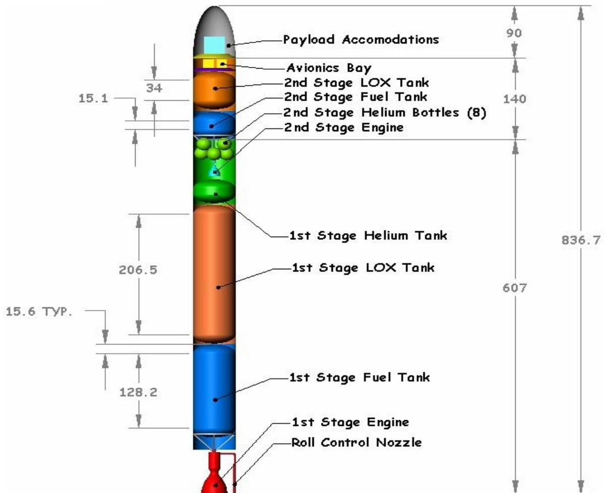
**Figure 1. Pressure-fed Two-Stage NLV**
