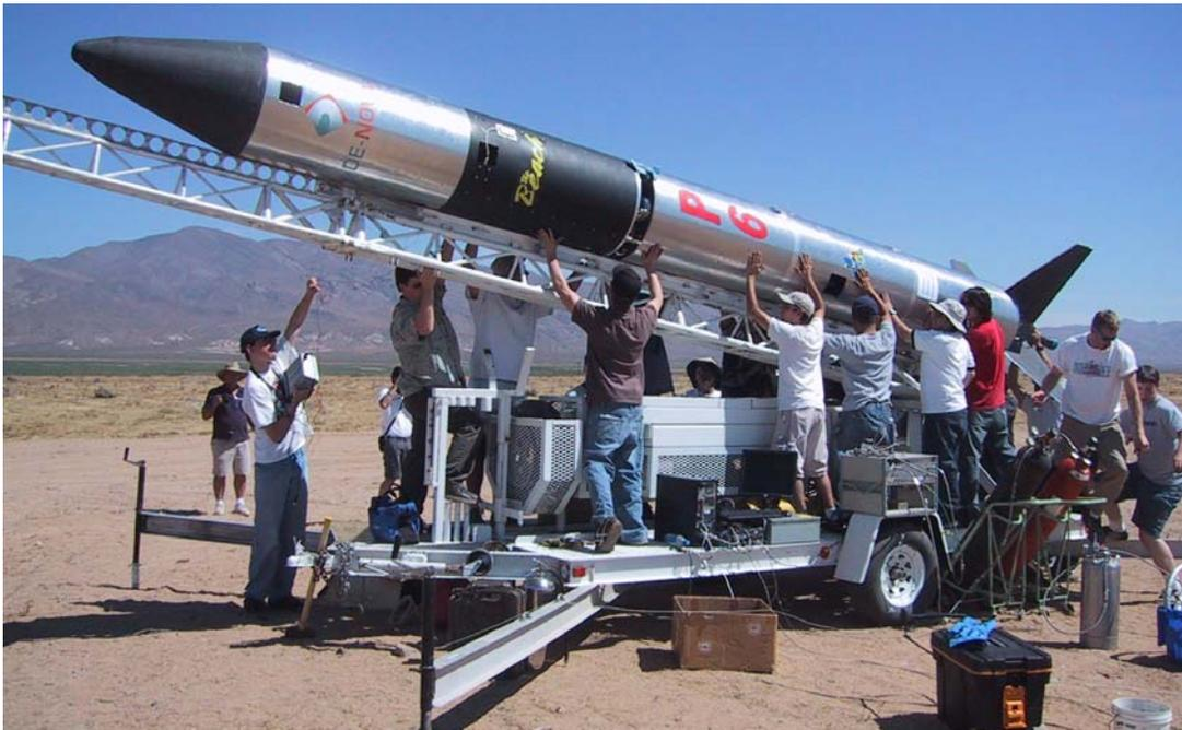
Figure 7. CSULB Students Integrating the P-6 With the Launch Rail
