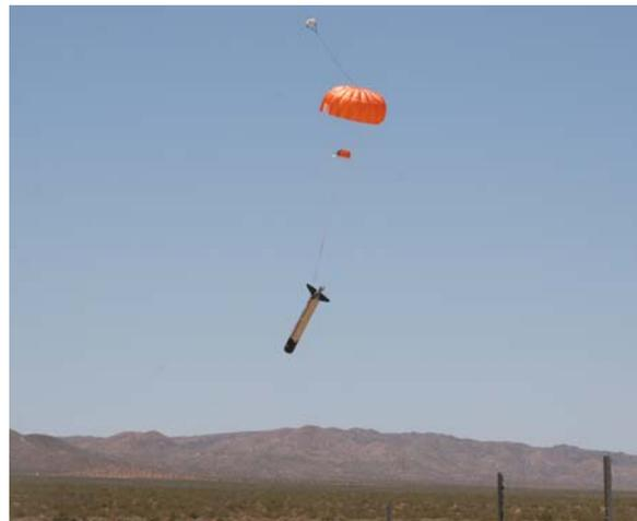
**Figure 13. P-6 First Stage/Interstage Assembly Just Prior to Landing**
