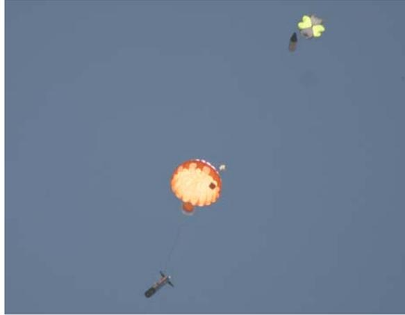
**Figure 12. Deployed Parachutes Shortly After P-6 Stage Separation**
