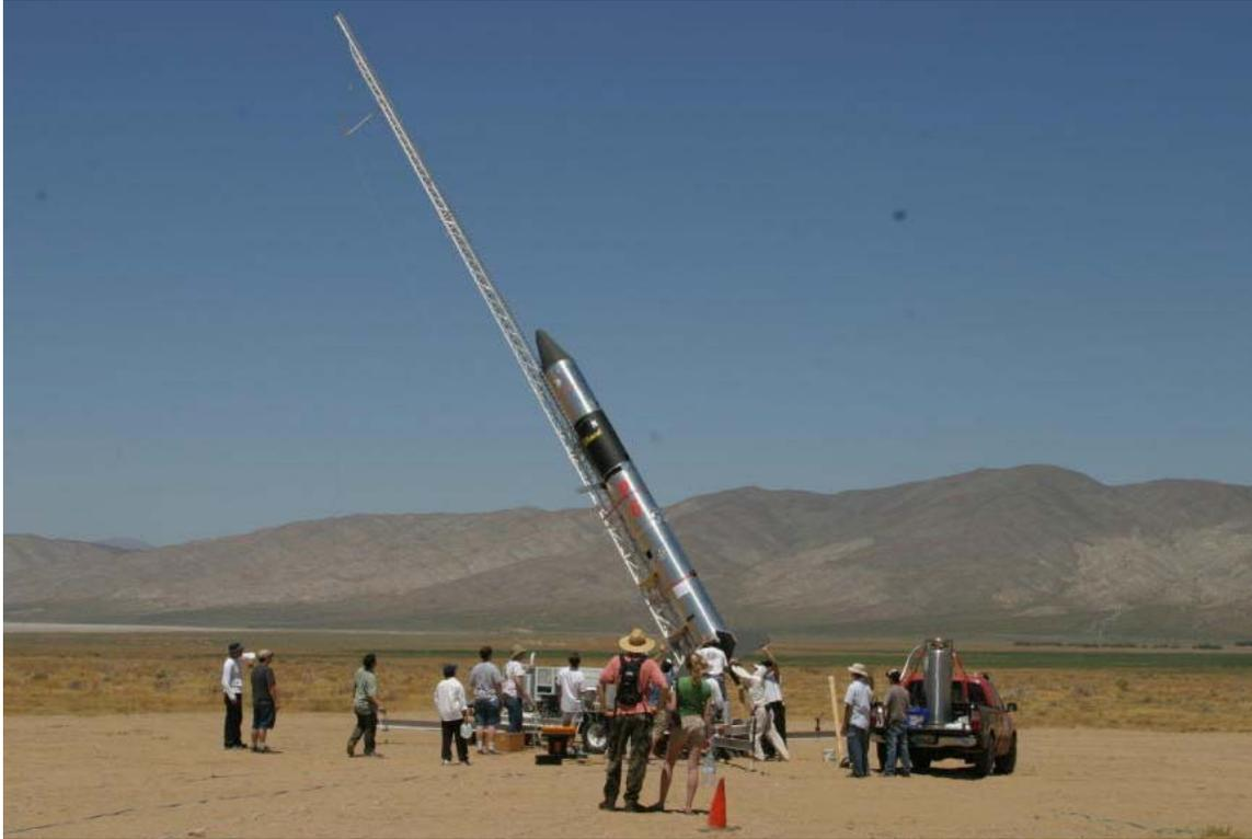
**Figure 8. P-6 being Erected into Launch Position**
