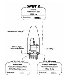
Fig. 3 – ASAP4 configuration for 6 micro-satellites
