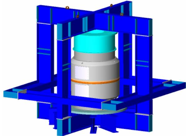
Figure 16. CASPAR structure in qualification load frame
