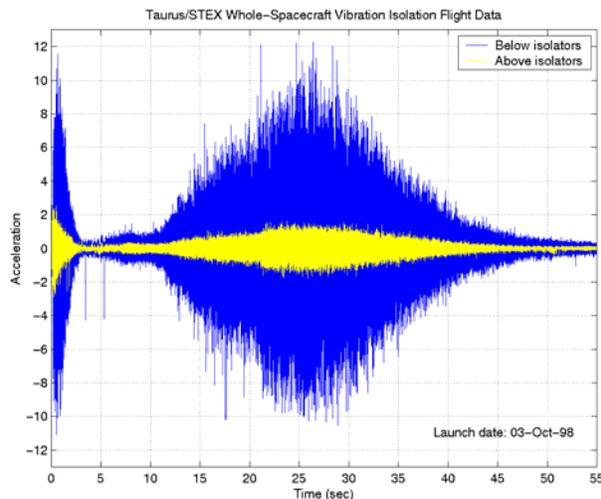
Figure 11. STEX flight data, below and above isolators
