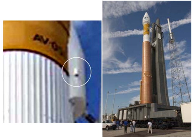
Figure 3. RocketCam Camera Attached to Atlas V.
