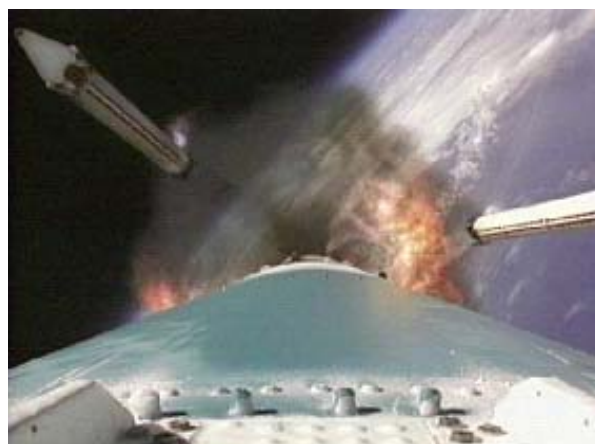
Figure 1. RocketCam View of Delta II SRM Sep.
