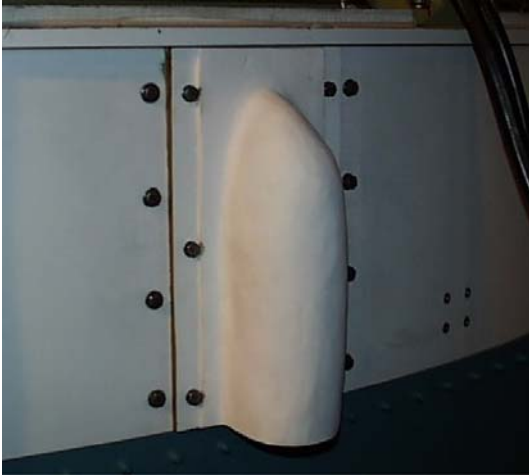
Figure 5. RocketCam Camera Pod on Delta II Mini-Skirt.
