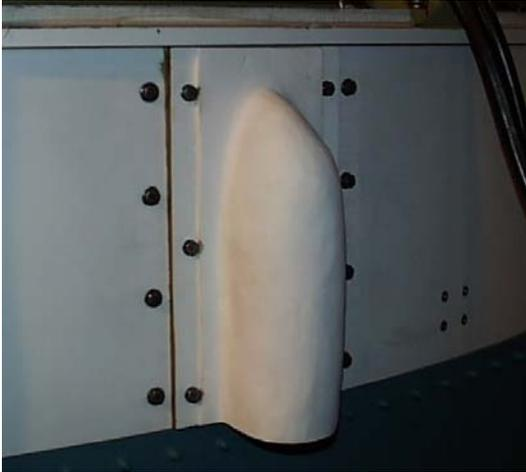
**Figure 5. RocketCam Camera Pod on Delta II Mini-Skirt.**
