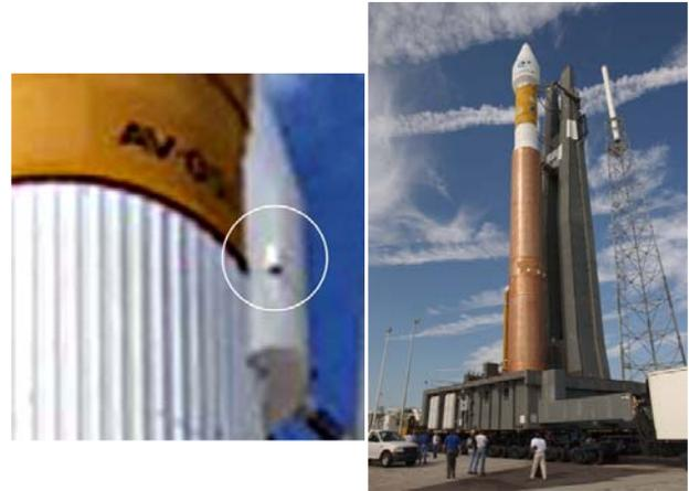
**Figure 3. RocketCam Camera Attached to Atlas V.**
