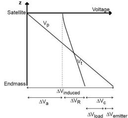
Figure 1. Tether voltage and plasma voltage along the tether length.
