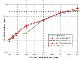
Figure 2. Simulated orbital Lifetime for a CubeSat satellite without deployables from a given initial circular orbital altitude.
