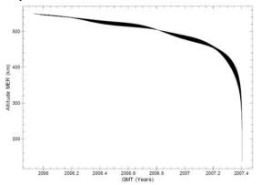
**Figure 9.** Simulated decay profile for a initial 550km sun-synchronous orbit (97.58° inclination) orbit.
