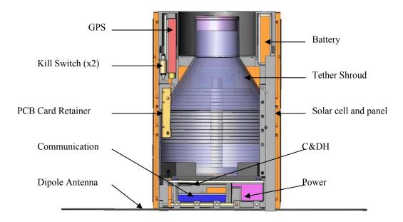
Figure 14: BarnacleSat Architecture and Subsystems.
