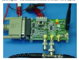
Figure 15: Communication System Prototype - Chipcon CC1000 Development Board.
