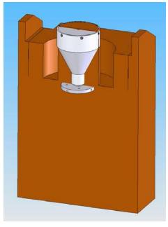
Figure 5. Rendered drawing of a CubeSat/RocketPod class nanoTerminator™ module. The device requires a 54.5mm by 38 mm diameter envelope, with a mass of less than 100 grams. This module fits nicely within the extended 'neck' volume of a standard RocketPod satellite, which is shown on the right.
