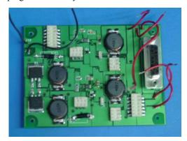
Figure 16: 5V Regulator, Test Board
