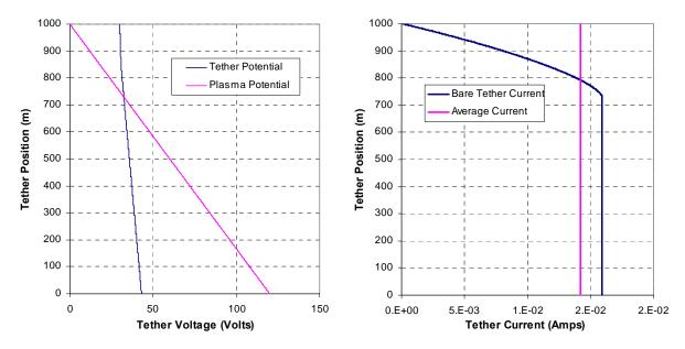
Figure 3. Voltage and current profiles of a 1km fully bare electrodynamic tether operating in generator mode with a  $10\Omega$  load and a cathodic emitter with a  $\Delta V_c$ = -75 volts.
