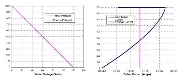
Figure 4. Voltage and current profiles for 1km fully bare contactor-less tether in low-earth orbit operating in deorbit (generator) mode.
