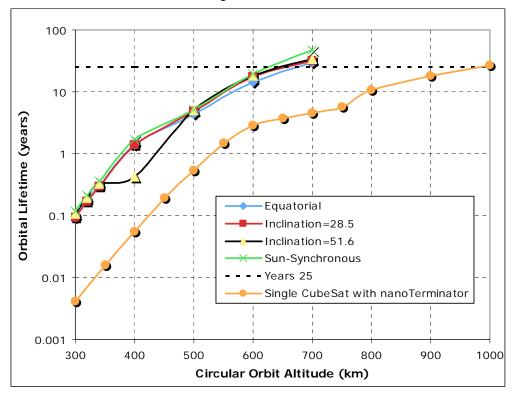
Figure 8. Simulated orbital Lifetime for a single CubeSat satellite without deployables from a given initial circular orbital altitude, as compared to a single CubeSat with a 100m nanoTerminator<sup>™</sup> contactorless deorbit tether system.
