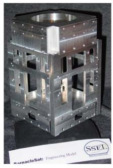
Figure 13: BarnacleSat Structure Engineering Model
