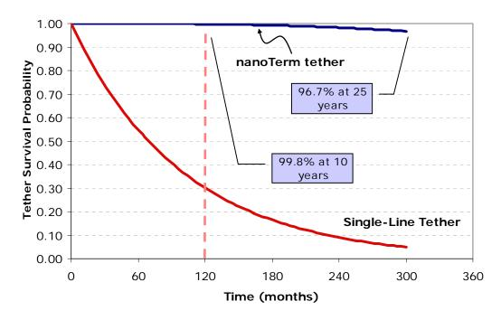
Figure 7. The predicted tether survivability of the nanoTerminator's tether and of an equivalent-diameter single-line tether over a 25 year MEO orbital lifetime.
