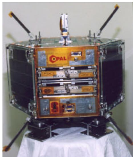
Figure 1. Opal [courtesy Stanford SSDL].
