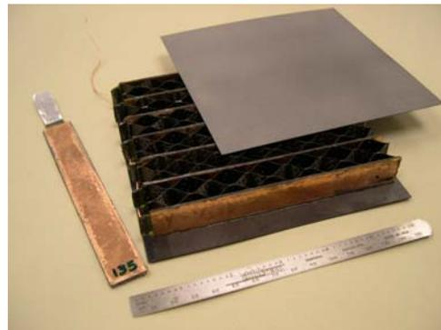
**Figure 1. Prototype Structural Battery Panel**
