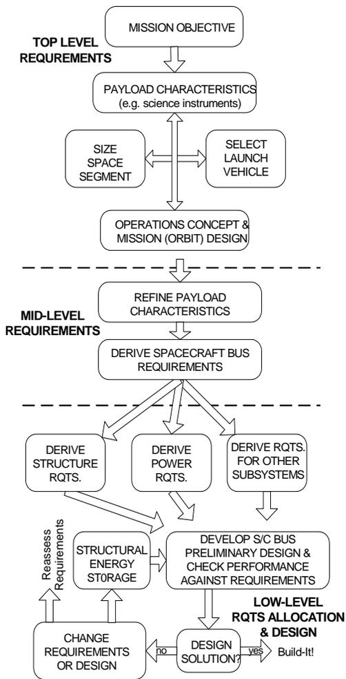
**Figure 5. Flow-down of requirements drives need for structural energy storage technology for some missions.**
