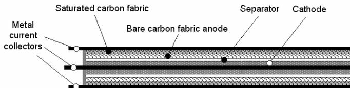
Structural Bicell with 2 carbon composite anodes, 1 cathode
