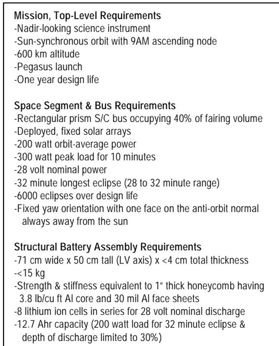
**Figure 6. Derivation of Key Requirements for Structural-Battery Side-Wall**
