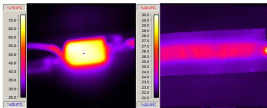
**Figure 3. Battery configurations that expose high surface area allow operation at lower temperatures than compact spiral-wound or prismatic designs.**
