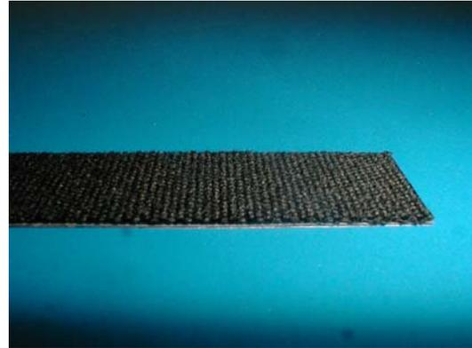
**Figure 4. Dual-function carbon composite ultracapacitor electrode**
