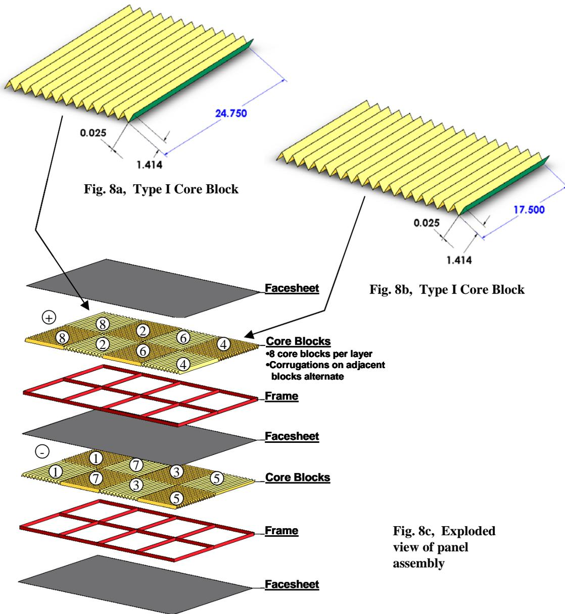
**Figure 8, Corrugated, electrochemically active subassemblies are layered to form 50 cm x 70 cm x 2.3 cm sandwich panel**
