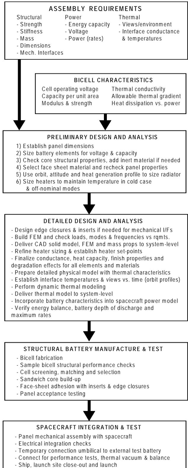
**Figure 7. Flow Shows Structural Battery as Part of a Spacecraft Development Process**
