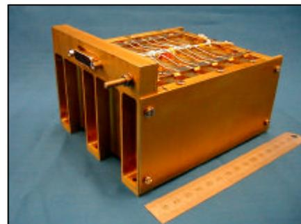
**Figure 16 – The final PROBA battery**
