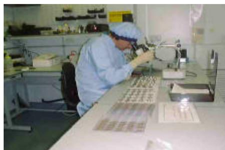
**Figure 4 Cell Destructive Physical Analysis**
