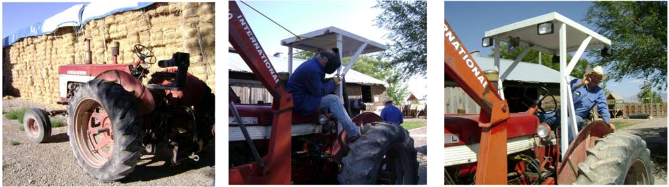
Figure 3. Shade structure added to tractor.
