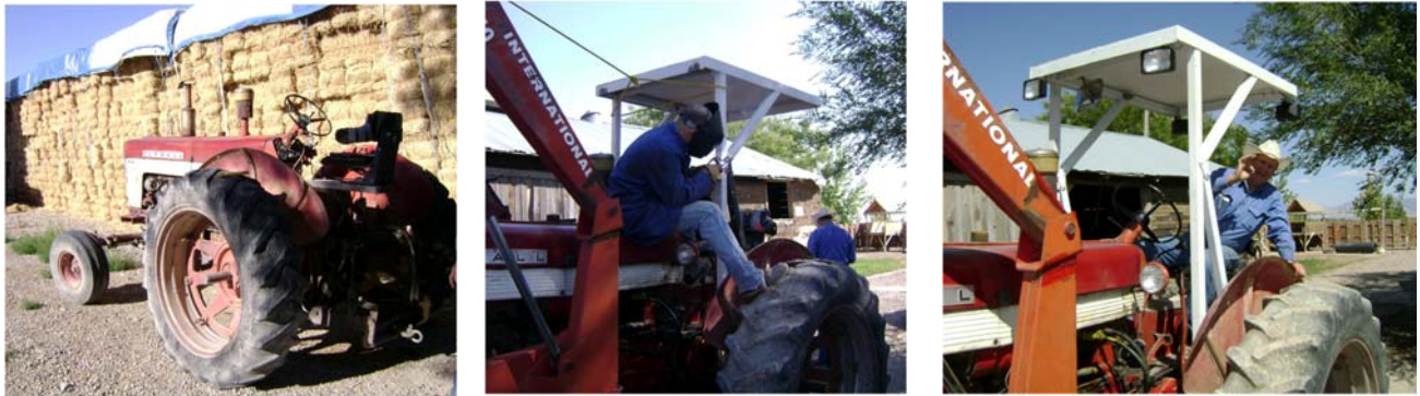
Figure 3. Shade structure added to tractor.
