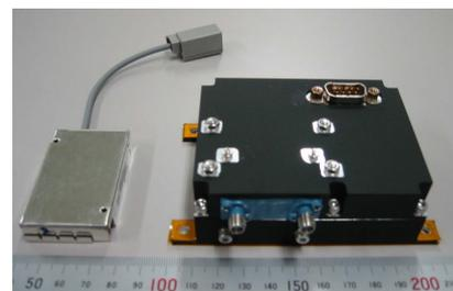
**Figure 1. Left : Automobile-Navigation GPS Receiver CCA-370HJ
