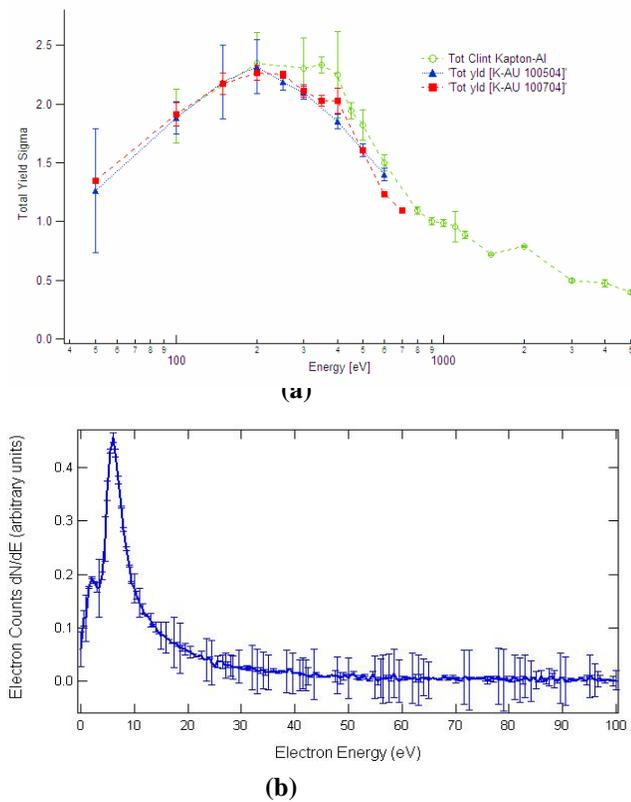
**Figure 4.** (a) Total yield data for 8  $\mu\text{m}$  thick Kapton<sup>TM</sup> on Aluminum and 25  $\mu\text{m}$  thick Kapton<sup>TM</sup> on Gold, using the pulsed yield technique. (b) Electron emission spectrum of 25  $\mu\text{m}$  thick Kapton<sup>TM</sup> on Au.
