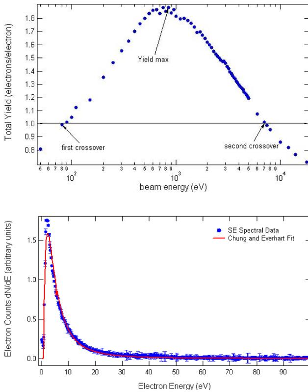
**Figure 1.** Electron emission from polycrystalline Au. (a) The total electron yield curve as a function of incident electron energy. Note the logarithmic energy axis. (b) Electron emission spectrum, induced from a 400 eV electron beam. Visible in the spectrum is the SE peak at 2.3 eV. The fit is based on Eq. 7 from the Chung and Everhart [8] model of electron emission spectra, with fitting parameters  $k=(5.93\pm 0.01)\cdot 10^5$  eV<sup>3</sup> and  $\varphi=(5.3\pm 0.1)$  eV.
