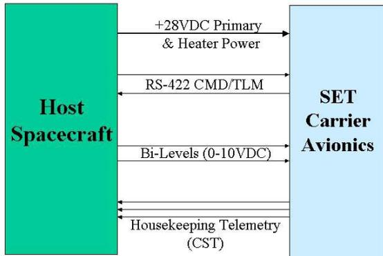
Figure 6-1 SET Carrier to Host Electrical Interface
