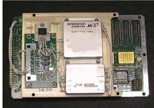
Figure 5.2-1 SET Carrier Processor Card
