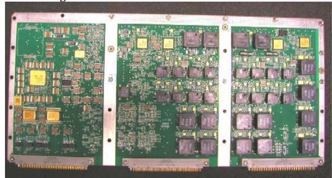
Figure 5.2-2: Power Control Card (PCC) Backside
