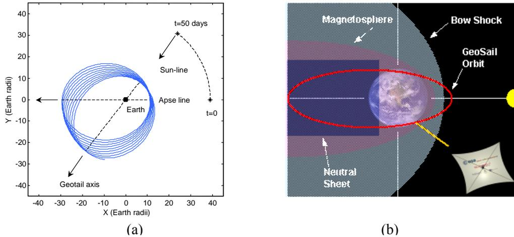
Figure 1: (a) Evolution of Elliptical Orbit at ~1 deg/day (b) SK Geosail Orbit
