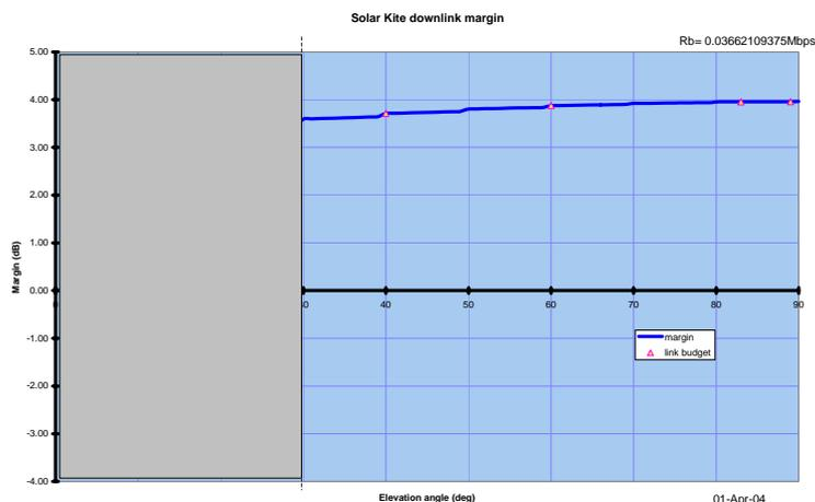
Figure 10: SK Downlink Margin at Apogee
