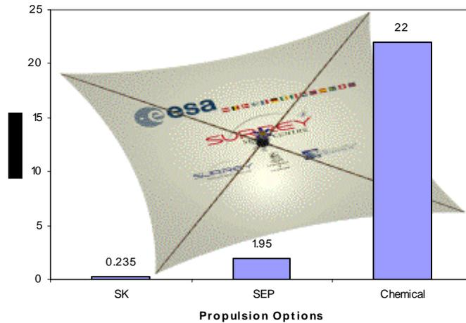
**Figure 2 – SK Propulsion Extra Mass Required**
