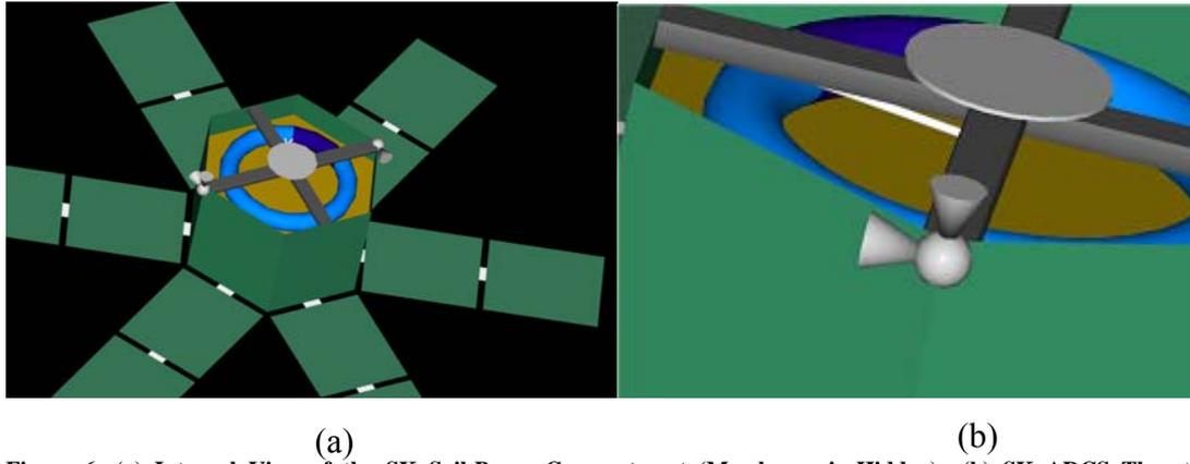
Figure 6: (a) Internal View of the SK Sail-Boom Compartment (Membrane is Hidden) (b) SK ADCS Thrusters (Membrane is Hidden)
