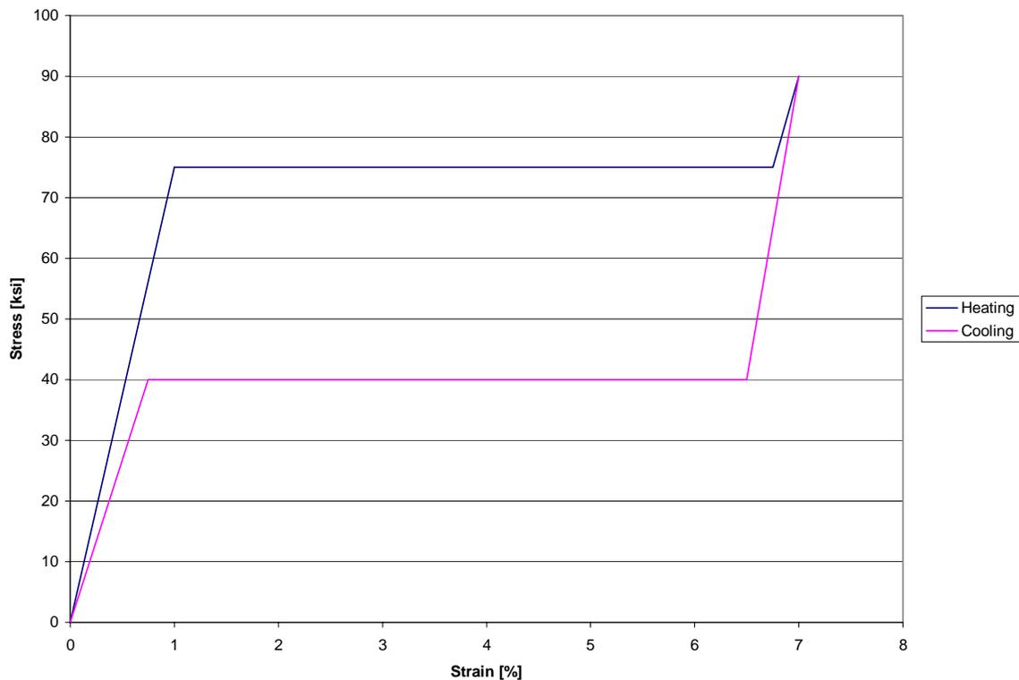
**Figure 2** Approximate stress-vs.-strain curve for NiTi shape memory alloy
