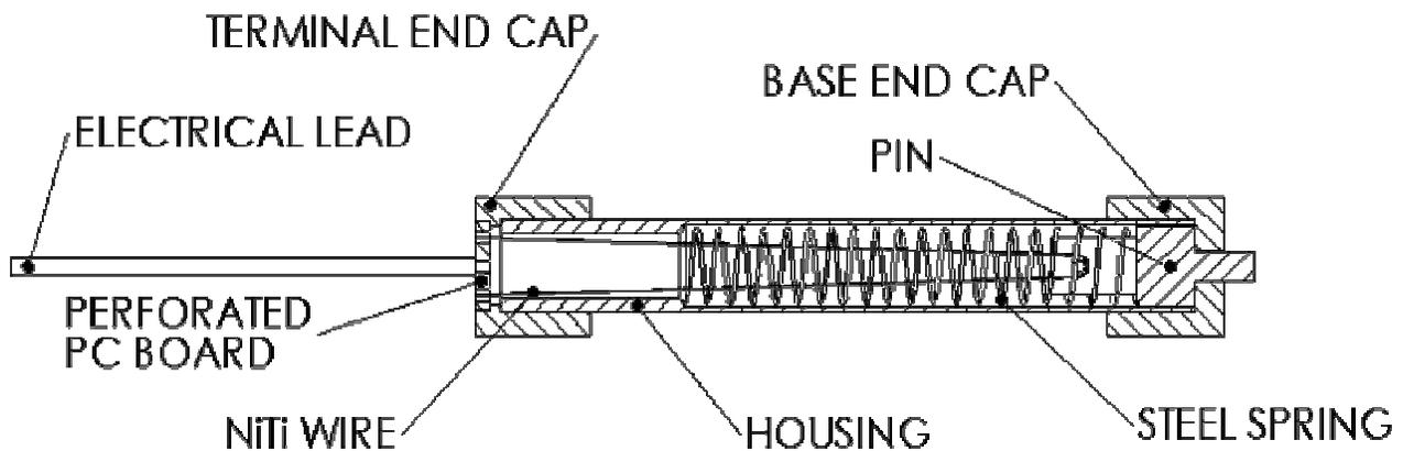
**Figure 5** Conceptual design of NiTi pin puller
