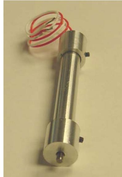
**Figure 4** Conceptual design prototype of NiTi pin puller
