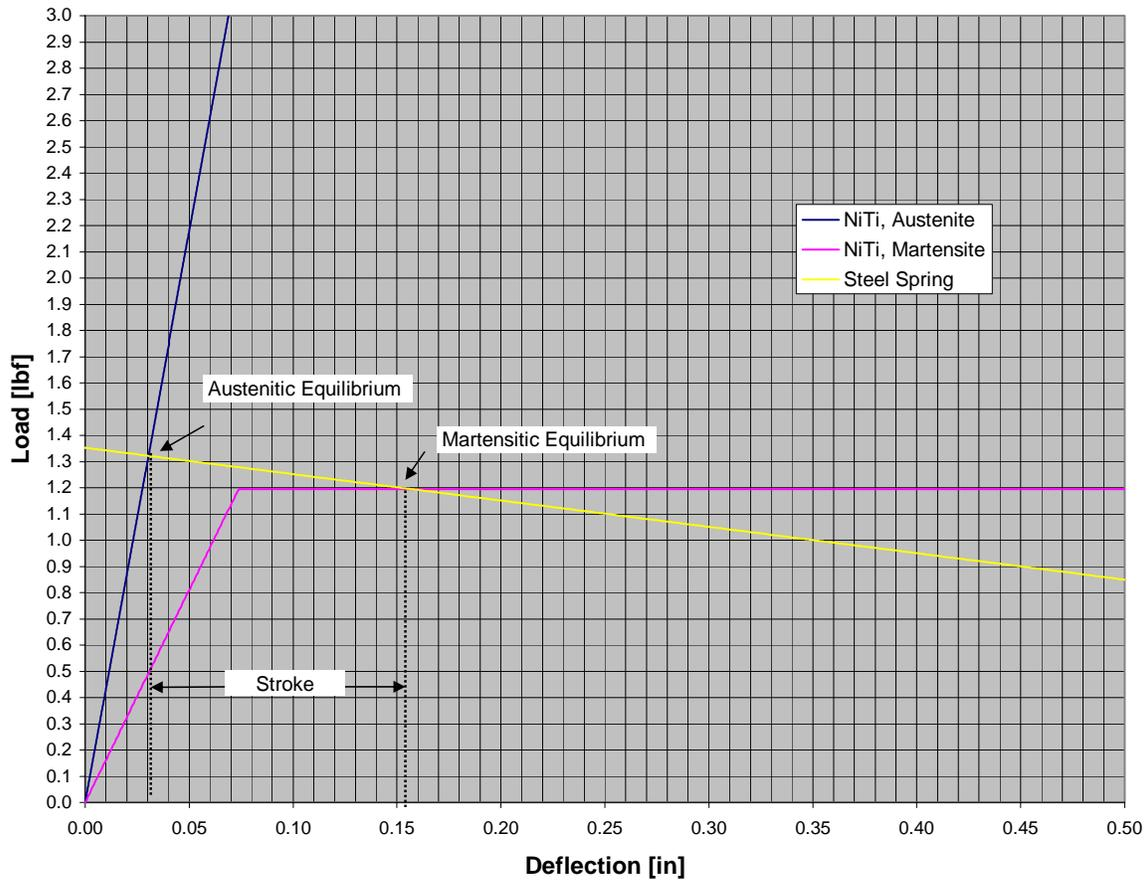
**Figure 3** Mechanical response of LionSat pin-puller
