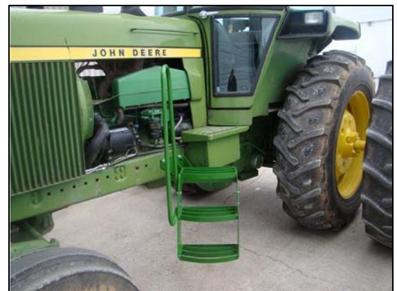
Figure 3. Additional tractor steps.
