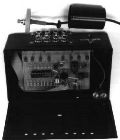
Fig. 4. Internal details of the Control Box and disassembled Push Button Switch.
