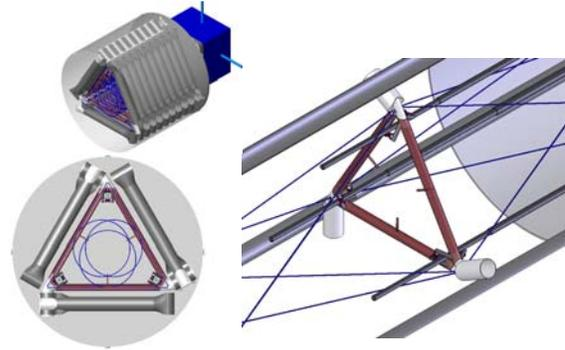
**Figure 9: Proposed FalconSat-3 EMC Truss Boom**
