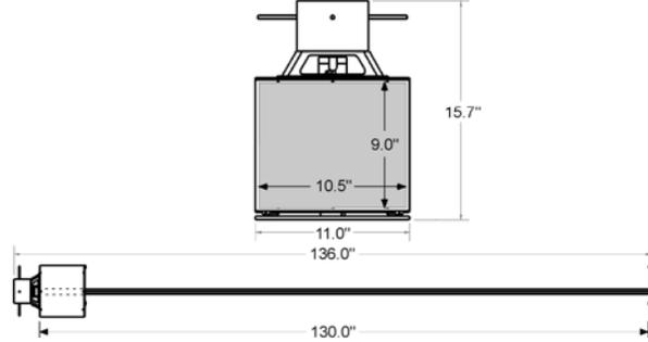
Figure 6: Packaging volume and deployed length.
