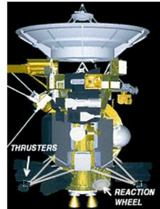
**Figure 1: Typical 3-Axis Attitude Control System.**
