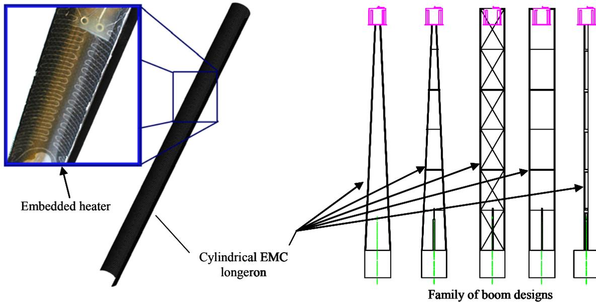
**Figure 4: Family of EMC boom configurations that share common EMC longeron components.**
