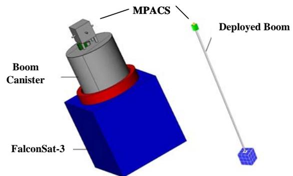
**Figure 5: Spacecraft layout and deployed boom.**
