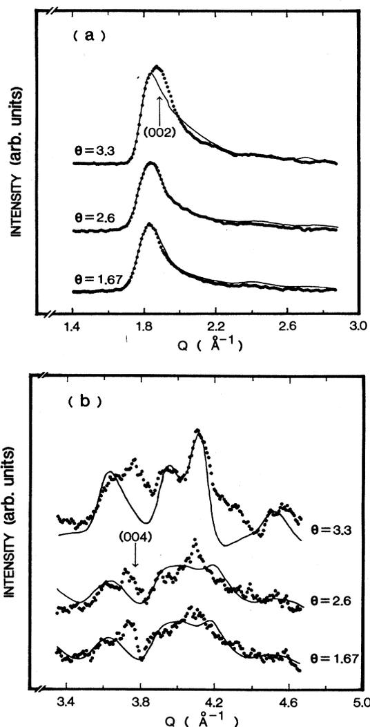
FIG. 3. Coverage dependence of the diffraction patterns below 11 K at coverages near crystallization of the bilayer: (a) low- $Q$  region and (b) high- $Q$  region. At each coverage, the diffracted neutron intensity has been scaled to the same number of monitor counts in the incident beam. The same solid curve from Fig. 2(b) has been superimposed on the patterns at  $\Theta = 1.67$  and 2.60. The solid curve at  $\Theta = 3.3$  is calculated for the pinwheel model of the bilayer in Fig. 7(b).
