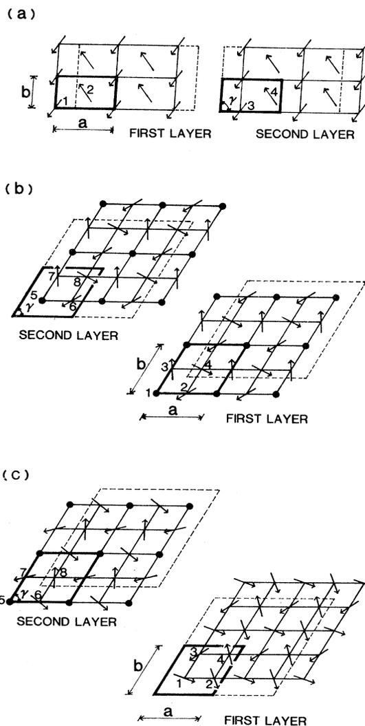
FIG. 6. Schematic diagrams of three bilayer crystal models: (a) herringbone bilayer, (b) pinwheel bilayer, and (c) herringbone first layer-pinwheel second layer. The azimuthal orientation  $\phi$  and tilt angle  $\beta$  of the molecules are measured as in Fig. 1.
