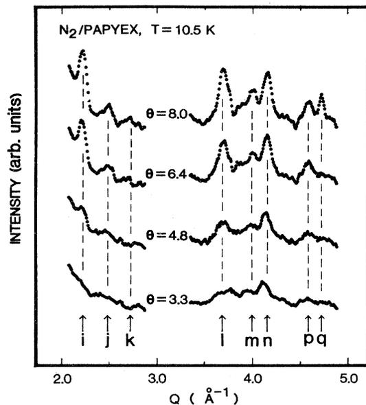
FIG. 4. Coverage dependence of the diffraction patterns at 10.5 K above  $\Theta=3.30$  layers. At each coverage the diffracted neutron intensity has been scaled to the same number of monitor counts in the incident beam. The letters correspond to the positions of the bulk  $\alpha$ - $N_2$  peaks as follows:  $i=(200)$ ,  $j=(102)$ ,  $k=(112)$ ,  $l=(113)$ ,  $m=(203)$ ,  $n=(213)$ ,  $p=(104)$ , and  $q=(114)$ .
