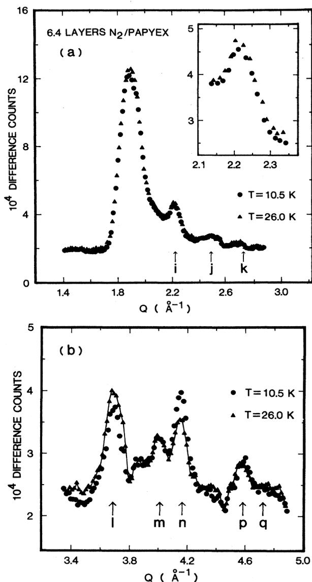
FIG. 8. Diffraction pattern of the 6.4-layer film at temperatures of 10.5 and 26.0 K: (a) low- $Q$  region and (b) high- $Q$  region. Inset in (a) shows with greater sensitivity the temperature independence of the peak labeled *i* corresponding to the bulk (200) peak of  $\alpha$ -N<sub>2</sub>. The labeling of the other peaks is the same as in Fig. 4. The solid curve in (b) is a guide to the eye through the high-temperature points.
